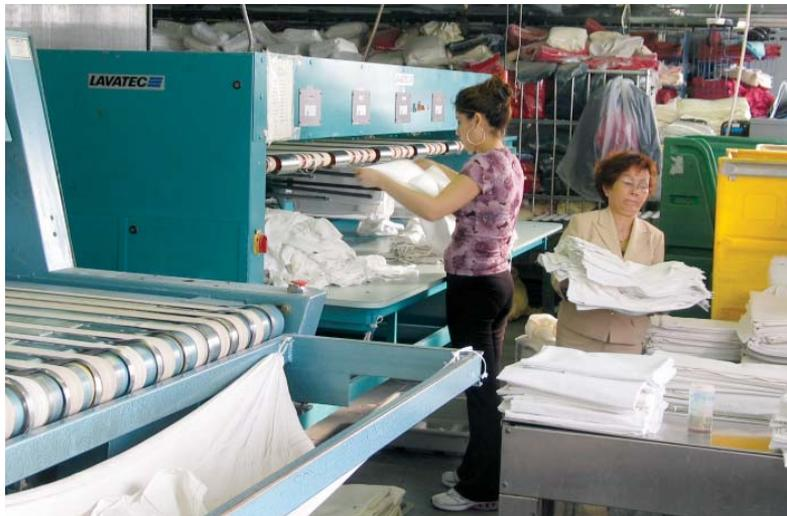
Ironers should receive periodic lubrication by running a wax cloth through the ironer every two hours. A wax cloth with a barrier flap is better because it won't let wax become embedded in the padding.
