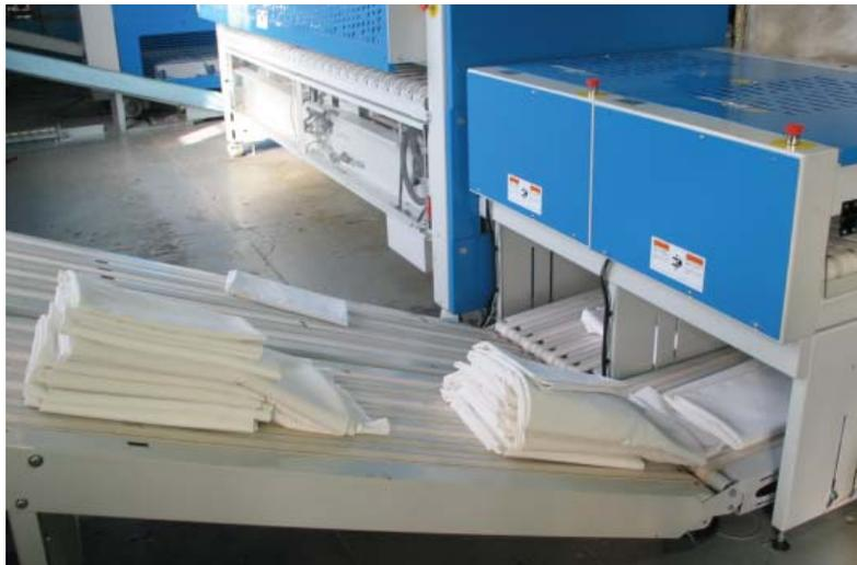
For quality results, it's important that finishing speeds increase from start to finish. That means the pace should increase 5%-10% from the feeder to the ironer and into the folder.
